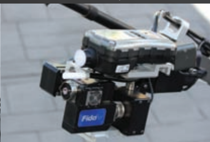
Lower Explosive Limit (LEL) O 2 Four Gas Sensor and Explosive Detector
